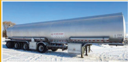
UNIT 10344 – 2004 REMTEC 57,000 Lts petroleum, 6 compts, bottom loading vapor recovery, auto steer, very clean solid unit. Price includes all new inspections.
