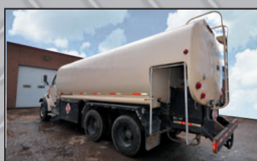
2007 STERLING FUEL DELIVERY UNIT C/W 20,000 L, 3 Compartment Pop Model Tank, 2 Sets Of Equipment And Midcom Registers, 5 yr/1 yr Inspect, Truck Newly Certified/Safetied. 765207
