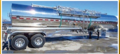
UNIT 10376 – 2017 NEW TREMCAR 7200 USG, DOT 407, 2 compt stainless insulated, equal split, very well spec'd. Call
