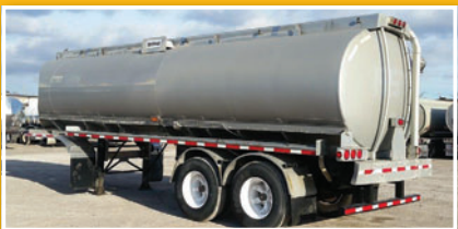
UNIT 10085 – 1998 HUTCH 28,000 Lts aluminum one compt non-code w/baffles, Newway air ride. 30ft O.A. length, new safety.
