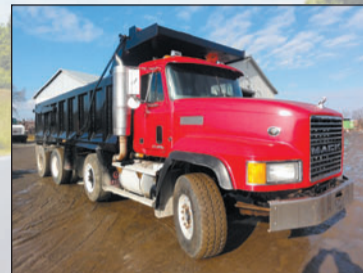
2001 MACK CL713 DUMP TRUCK E7 460XT; 18 SPD. EATON; 20 FRONT/20 STEER/LIFT/46 MACK RUBBER BLOCK REARS, 20'6" EXCAV. BOX, STK#229-07. -444437
