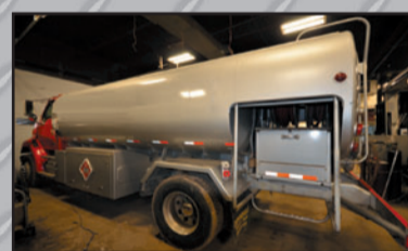
2002 STERLING L8000 c/w 13,000 L 4 Comp't Alum. Tank, Dual Pump/Meter, Midcom, Bottom Load, Vapor Recovery, New 5 yr/1 yr Inspect, New Truck DOT Insp./Certified, Stk#S812 502042
