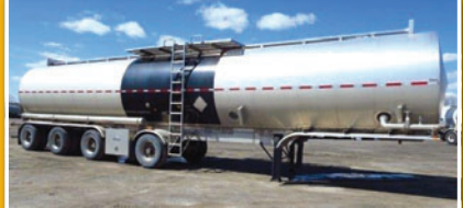
UNIT 10371 – 2014 TREMCAR 49,000 Lts, DOT-406 convertible, aluminum insulated, pump-off line, heat coils, stainless frame.
