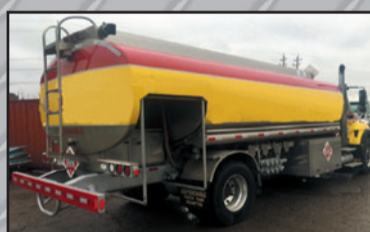
2004 INTERNATIONAL 7400 c/w 13,000 L 4 Comp't Alum. Tank, Dual Pumping/Metering, Midcom, Bottom Load RI, Vapor Recovery RI, New Tank 5 yr/1 yr Inspect, Truck Newly Certified/Safetied. Stk#S826 502041
